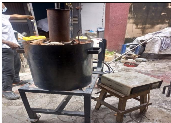
Figure 8 Pyrolysis Reactor used for Incineration Process
